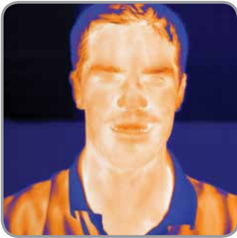
Figure 12. IR image from a 1024 × 1024 InSb detector camera
