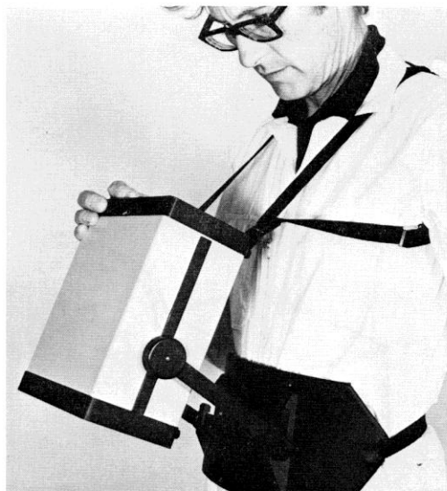
The carrying harness enables the operator to observe the thermal-picture display while standing or walking with the equipment.
