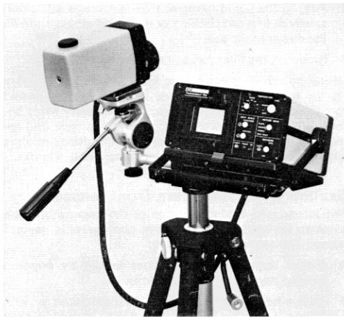
The tripod-platform provides an integrated IR-camera/display setup for fixed-site viewing.
