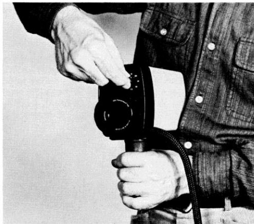
Selecting the temperature-range aperture setting on the front of the camera unit.
